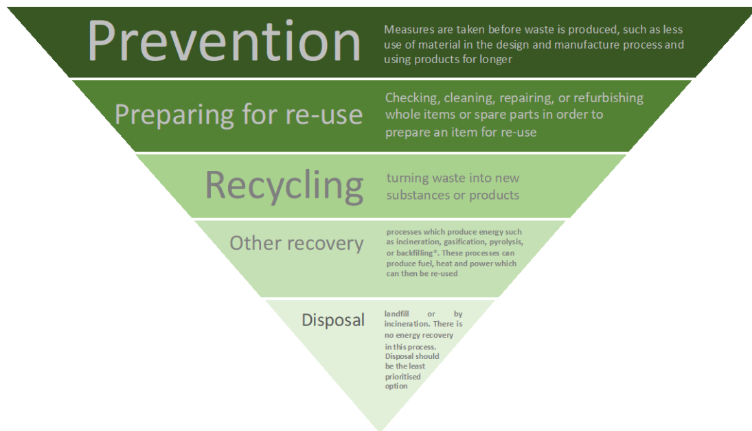
Figure 1: Waste hierarchy [*Gasification – reaction of waste with oxygen and/or steam, resulting in the production of carbon monoxide, carbon dioxide, and hydrogen. Pyrolysis – process of heating organic substances to above decomposition temperatures resulting in production of char and eventually ash. Backfilling – reclaiming excavated areas for landscaping purposes using non-hazardous waste as a substitute for non-waste materials. 11
